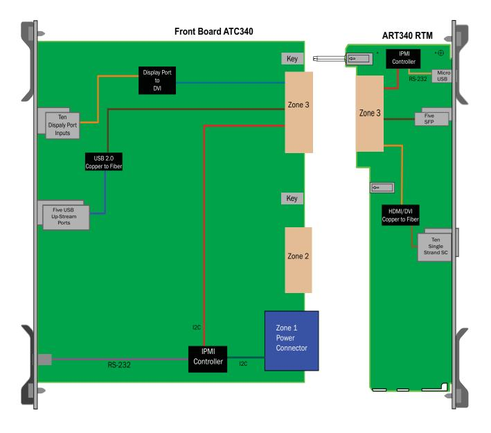
FIGURE 1. ATC340 Functional Block Diagram
